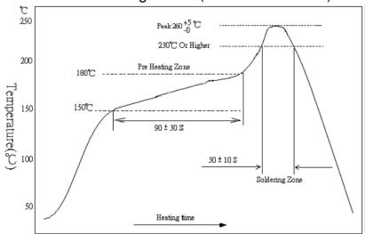
Remark: The peak temperature of soldering heat is 260 +5/-0  $^{\circ}$ C for 10 seconds
